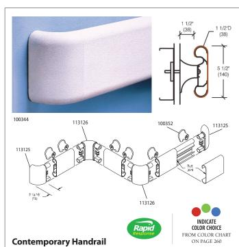
Contemporary Handrail is ideal for heavily-traveled areas. Rugged guard rail protects 5½" of wall surface and provides an optimum 1½" gripping area. Grip surface totally covers sturdy aluminum frame.
